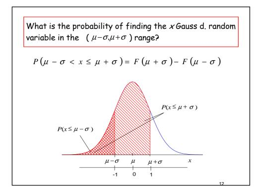
$$z_{lower} = \frac{\mu - \sigma - \mu}{\sigma} = -1 \qquad z_{upper} = \frac{\mu + \sigma - \mu}{\sigma} = 1$$
