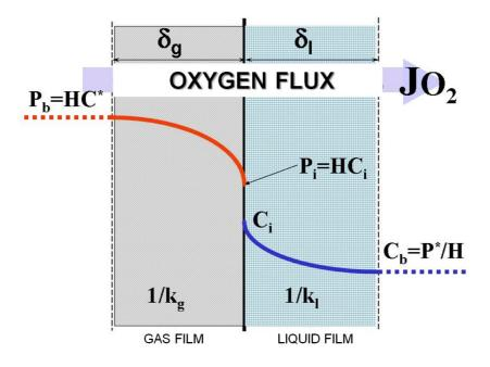
Fig.4.75.: Scheme of the two-film theory
