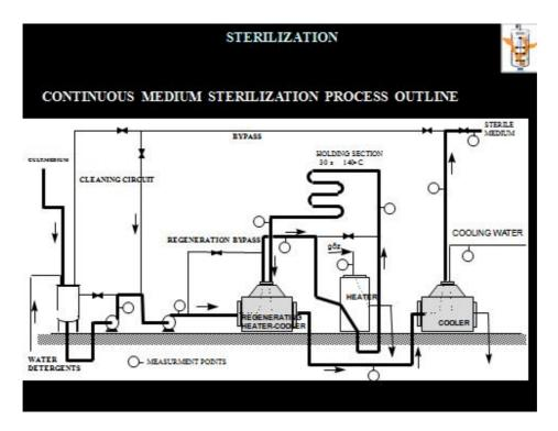
Fig. 4.151.: Siral heat exchanger continuous sterilization system
