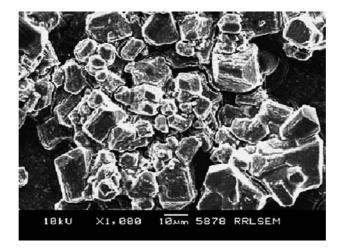
Fig 2.60.: Crosslinked enzyme crystals (CLEC)
