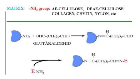
Fig 2.56.: Chemical immobilization with glutarealdehyde
