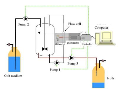
Fig 4.60.: Setup of a turbidostat
