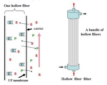
Fig 2.64.: Hollow fiber, UF membrane
