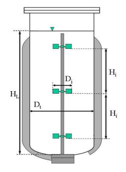
Fig 4.85.: Bioreactor with more mixing devices
