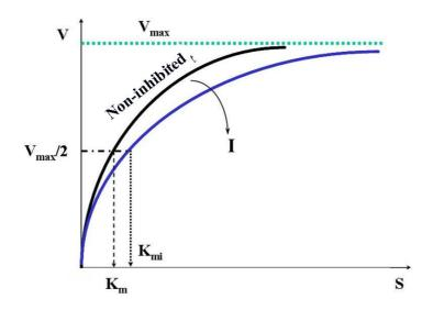
Fig.2.29.: V-S plot of competitive inhibition
