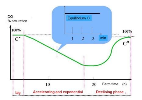
Fig. 4.77.: Equilibrium dissolved oxygen concentration in the time course of a batch fermentation.
