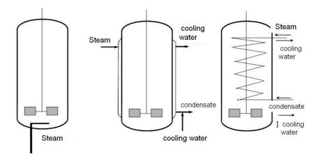
Fig. 4.147: Heating, cooling solutions
