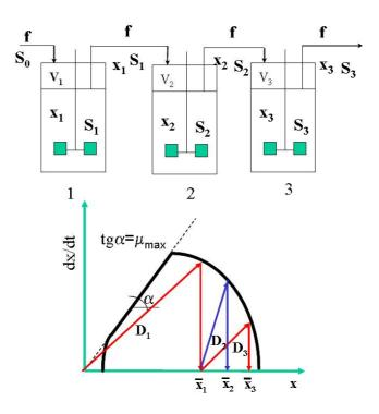
Fig.4.54.: Single stream multiple stage continuous system
