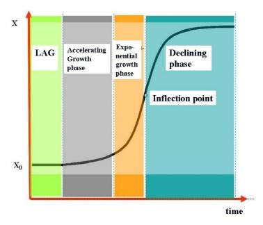
Fig 4.2.: Bach fermentation's real growth curve
