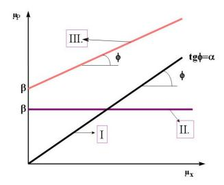
Fig 4.29.: Luedeking–Piret model of production
