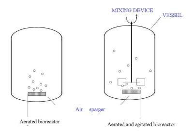
Fig 4.79.: Technical realization of aeration in bioreactors
