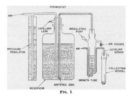
Fig. 4.41.: The "original chemostat" of Novick and Szilárd
