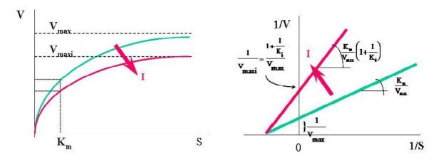
Fig 2.33: M-M and L-B plots of noncompetitive inhibition
