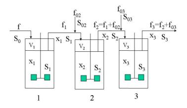
Fig 4.55.: Multistream multistage chemostat
