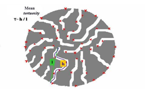
Fig 2.66.: Gel entrapped enzyme. Definition of tortuosity.
