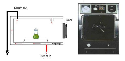
Fig.4.145.: Recently used sterilizer autoclave
