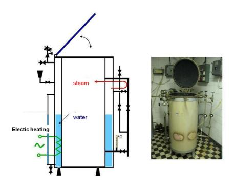
Fig 4.144: Conventional laboratory sterilizing autoclave
