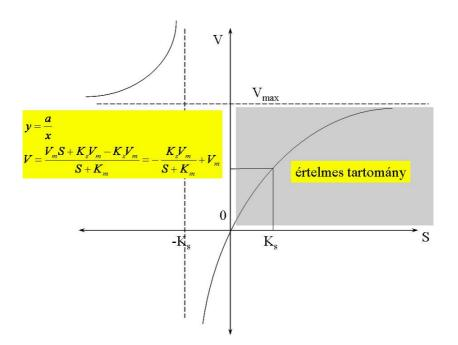
Fig.2.19.: M–M-equation is a transformed hyperbole
