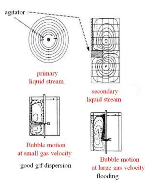
Fig 4.86.: Primary and secondary fluid streams and bubble movement in agitated reactors
