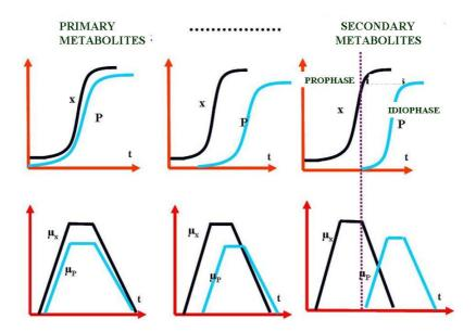
Fig 4.28.: Production types according Gaden
