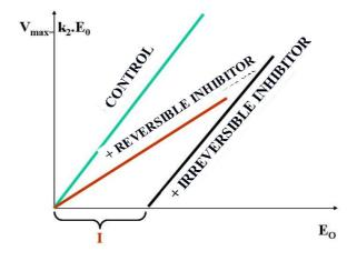
Fig 2.26.: Recognition of an irreversible inhibitor
