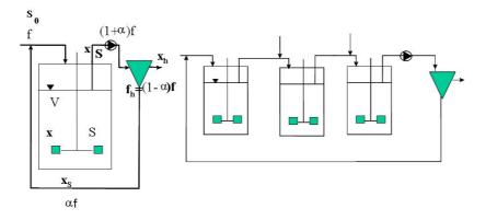
Fig 4.56: Cell retention and recycle
