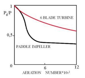
*Fig.4.89.: P<sub>s</sub>*/*P* depends on the aeration number
