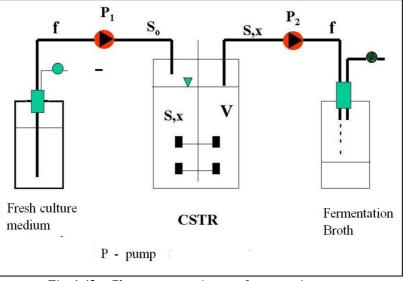
Fig 4.42.: Chemostat continuous fermentation setup
