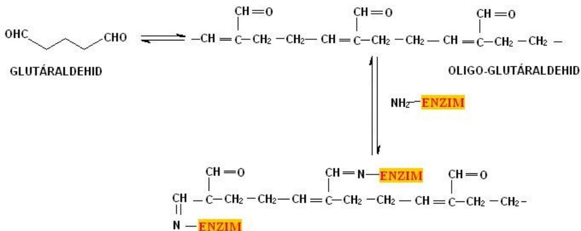
Fig 2.59. Crosslinking as an immobilization method
