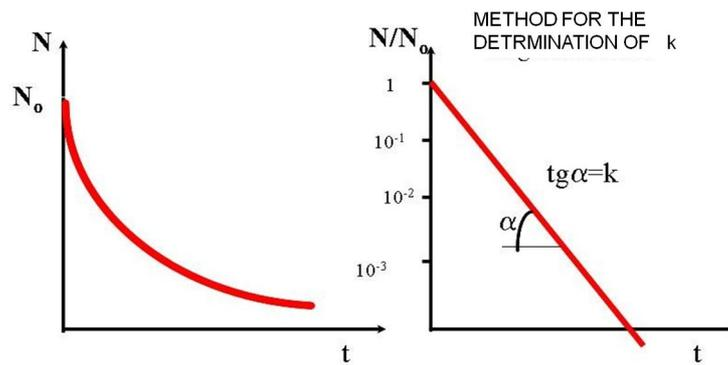
Fig 4.139.: Exponential heat decay. Determination of decay constant
