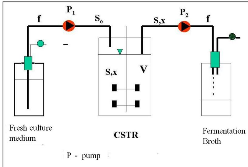
Fig 4.42.: Chemostat continuous fermentation setup
