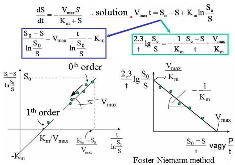
Fig2.20.: Linearization methods of the integrated M–M-equation
