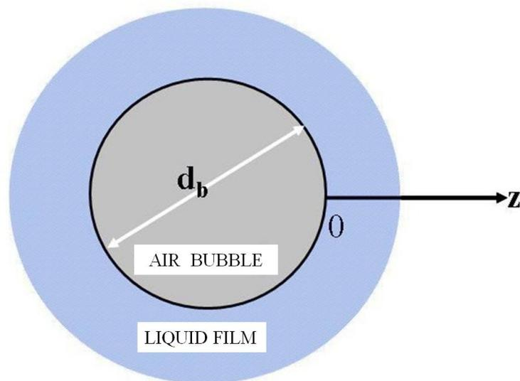
Fig 4.80.: One dimensional model of mass transfer from bubble.
