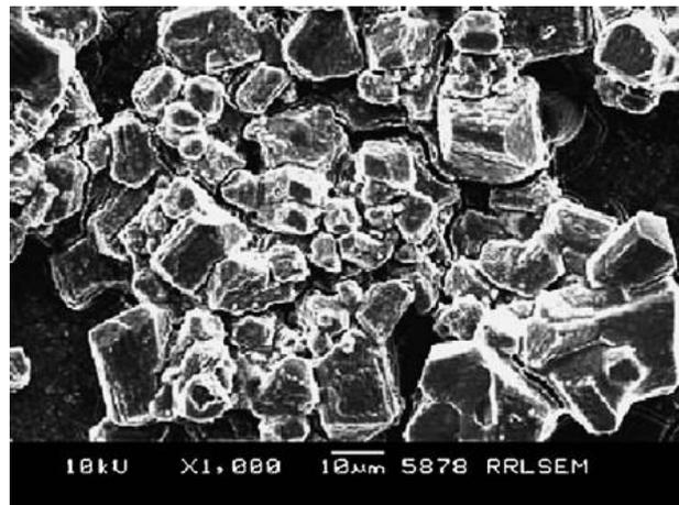
Fig 2.60.: Crosslinked enzyme crystals (CLEC)
