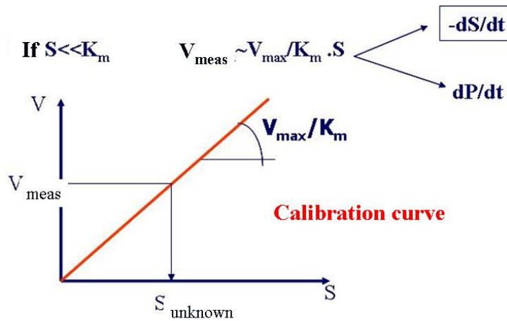
Fig 2.72.: Substrate determination on the basis of kinetic measurement.
