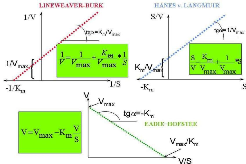
Fig2.21.: Linearizations of M–M-equation
