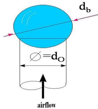
Fig.4.82.: Bubble evolution on an orifice
