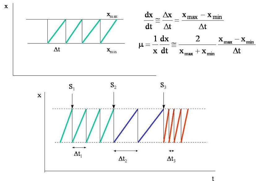
Fig. 4.59.: Turbidostat continuous fermentation and its use for optimization
