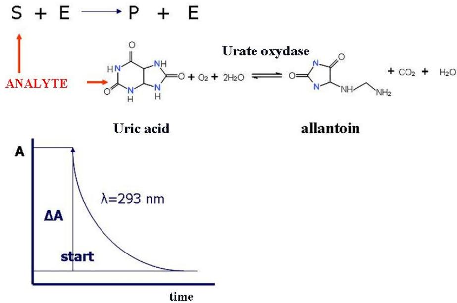
Fig 2.69.: Substrate determination with a reaction run to end point
