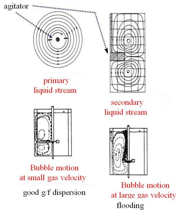
Fig 4.86.: Primary and secondary fluid streams and bubble movement in agitated reactors
