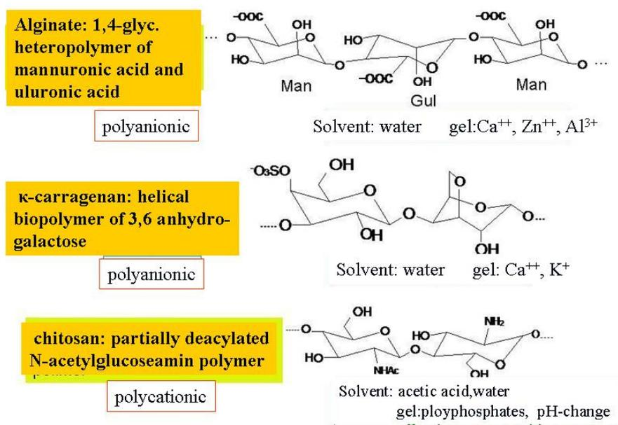
Fig 2.61. Gel forming polymers for enzyme immobilization
