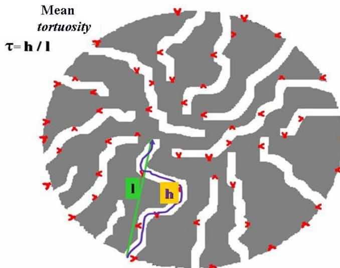
Fig 2.66.: Gel entrapped enzyme. Definition of tortuosity.
