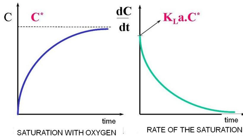
Fig 4.76.: Oxygen absorption: saturation and absorption rate
