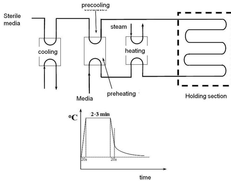
Fig. 4.149.: Sheet and plate heat exchanger continuous sterilization system
