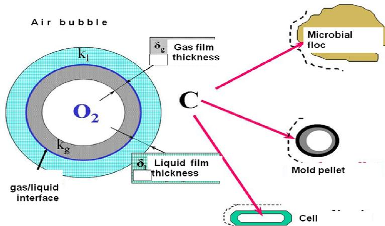
Fig 4.74.: Process steps of the oxygen absorption from a gas bubble and the uptake by the microbes.
