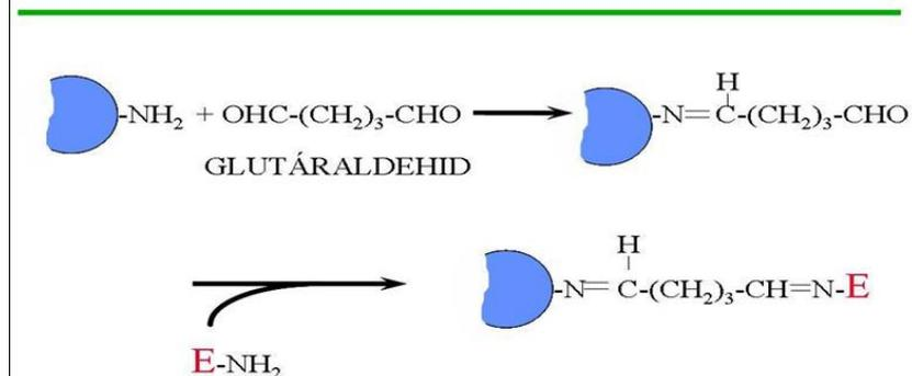
Fig 2.56.: Chemical immobilization with glutarealdehyde
