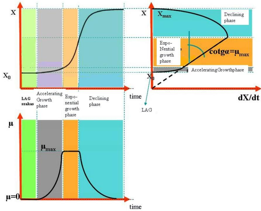
Fig 4.3.: Growth curve of batch fermentation and its primary kinetic representations
