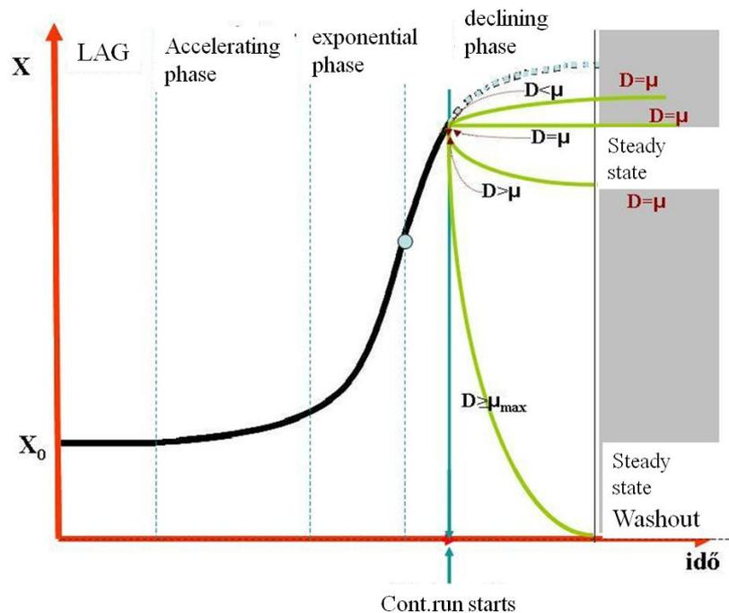
Fig 4.45.: Continuous fermentation starts as a batch one.
