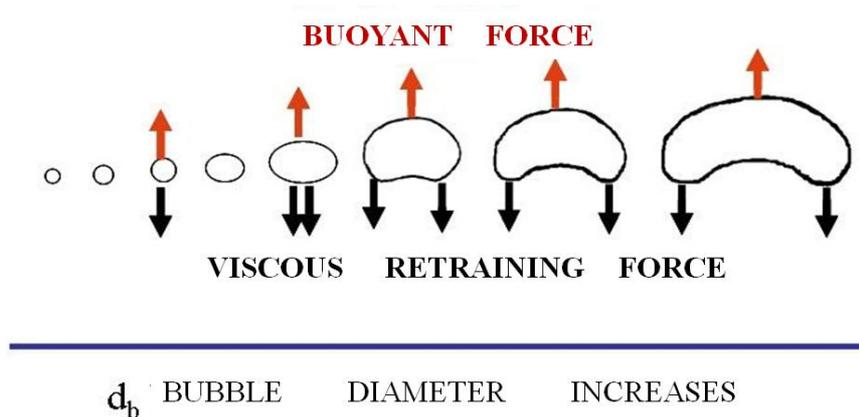
Fig 4.81.: Deformation of the bubble shape with the increasing diameter
