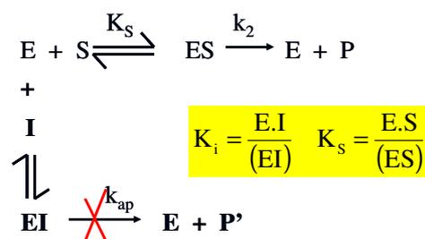
If  $k_{ap} > 0$ , then I is an *alternative substrate of E* and, P' is its alternative product. E.g., in case of hexokinase, glucose is the substrate and fructose may be an alternative substrate, the enzyme equally able to phosphorylate both.
