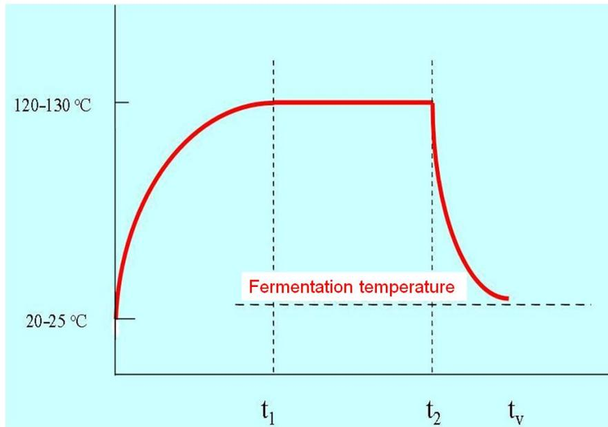
Fig.4.146.: Heat penetration curve
