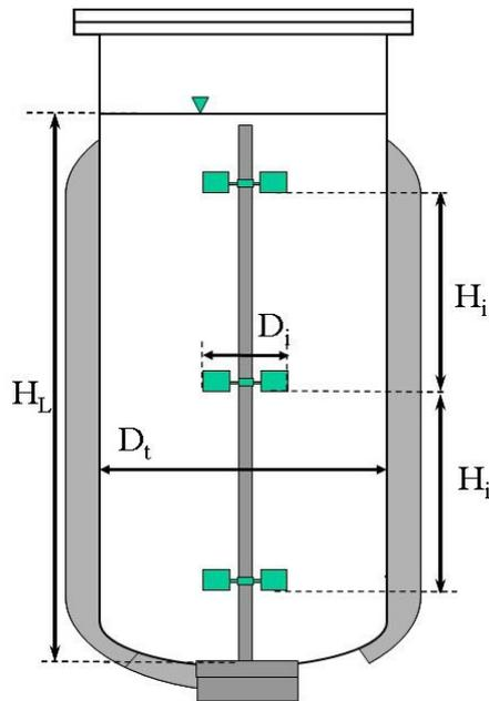
Fig 4.85.: Bioreactor with more mixing devices
