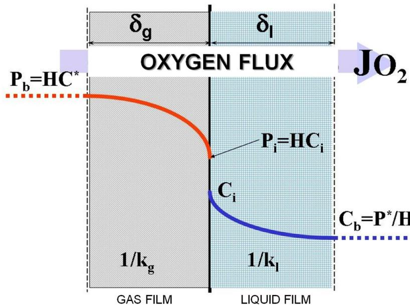
Fig.4.75.: Scheme of the two-film theory
