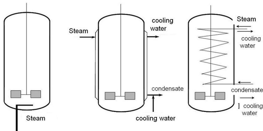
Fig. 4.147: Heating, cooling solutions
