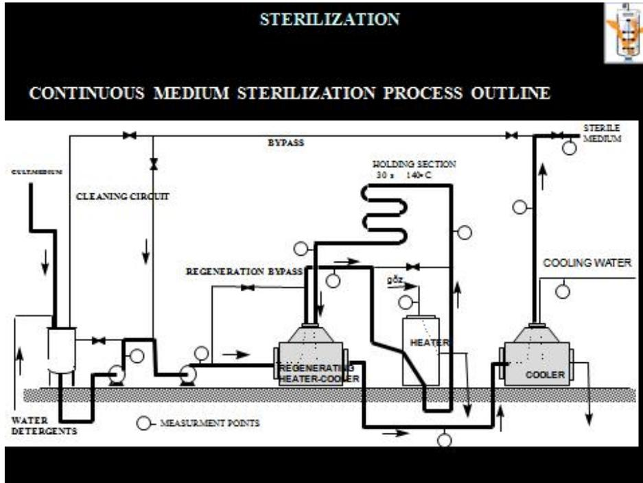
Fig. 4.151.: Spiral heat exchanger continuous sterilization system
