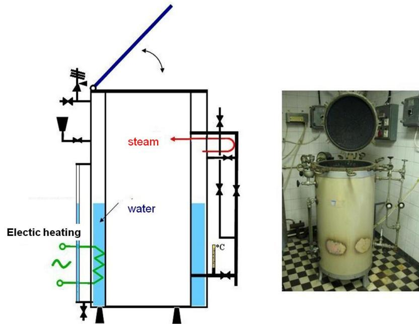
Fig 4.144: Conventional laboratory sterilizing autoclave
