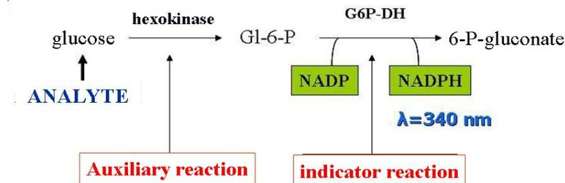
Fig 2.70.: Substrate determination with auxiliary reaction
