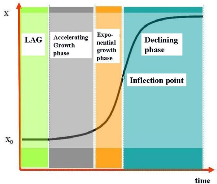
Fig 4.2.: Batch fermentation's real growth curve
