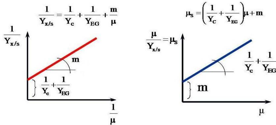
Fig 4.19.: Graphical determination of maintenance coefficient
