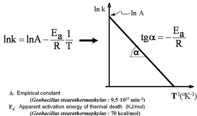
Fig. 4.140.: Temperature dependence of thermal decay constant
