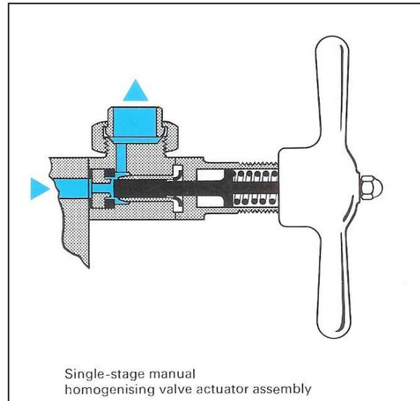
The discharge pressure is controlled by a handwheel assembly, which, through a springloaded valve rod, positions the valve, in relation to the valve seat. During disruption, the cell suspension passes between the valve and its seat and impinges on an impact ring.
