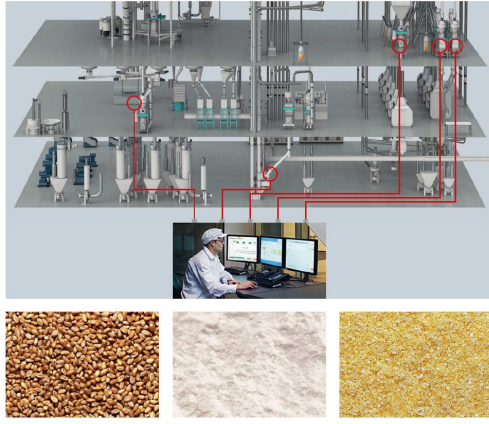
Online measurement of whole grain, flour, and semolina
