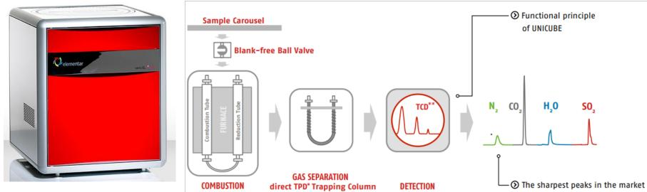
Simultaneous C, H, N, S determination is based on high-temperature (up to 1200°C) combustion of the sample in the oxygen stream. Gaseous products of combustion ( $N_2$ ,  $CO_2$ ,  $H_2O$  a  $SO_2$ ) are purified, separated and finally determined by TCD. Typical samples are organic chemicals but lot of inorganic matters can be analyzed as well.
