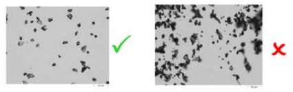
Illustration of the importance of sample dispersion for automated particle imaging.
