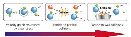
Illustration of the three dry powder dispersion mechanisms with increasing energy/ aggressivity.
