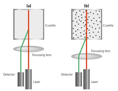
(a) For small particles, or samples at low concentrations, it is beneficial to maximize the amount of scattering from the sample. As the laser passes through the wall of the cuvette, the difference in refractive index between the air and the material of the cuvette causes 'flare'. This flare may interfere with the signal from the scattering particles. Moving the measurement position away from the cuvette wall towards the centre of the cuvette will remove this effect.
