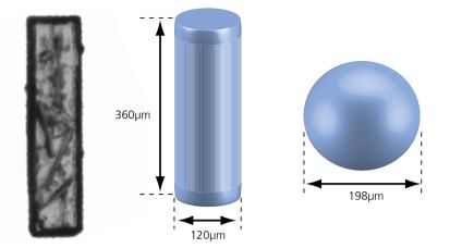
Illustration of the volume equivalent rod and sphere of a needle shaped particle.
