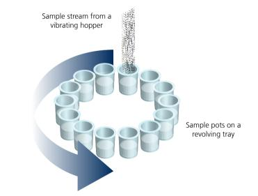
Illustration of a spinning riffler device.
