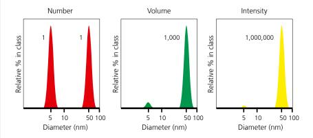
Example of number, volume and intensity weighted particle size distributions for the same sample.
