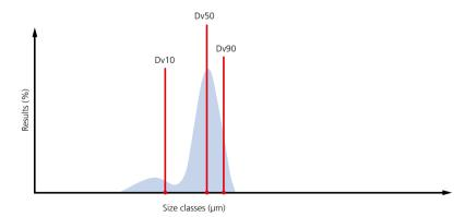
Illustration of the Dv10, Dv50 and Dv90 on a typical particle size distribution where a significant proportion of fines are present.
