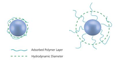
Illustration of the reported hydrodynamic diameter in DLS being larger than the 'core' diameter.
