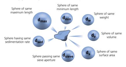
Illustration of the concept of equivalent spheres.
