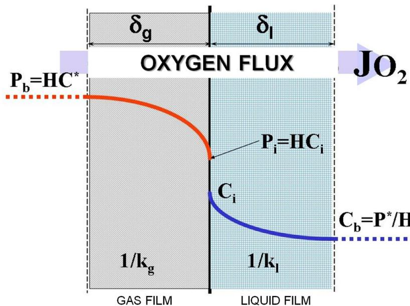
Fig.4.75.: Scheme of the two-film theory
