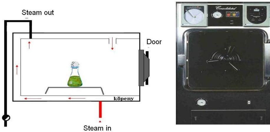
Fig.4.145.: Recently used sterilizer autoclave
