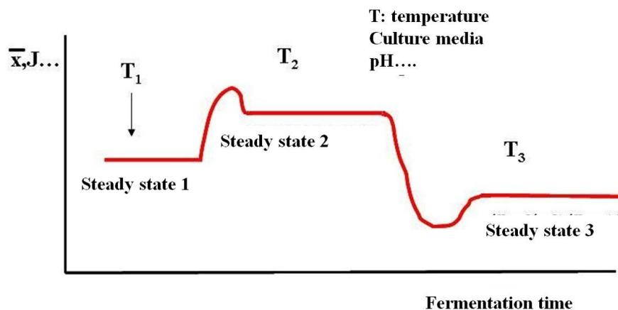
Fig. 4.53. Using chemostat for optimization
