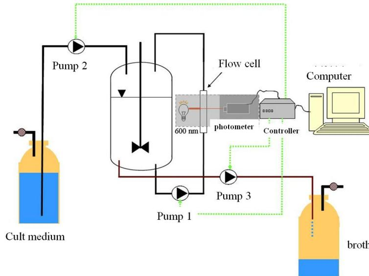
Fig 4.60.: Setup of a turbidostat
