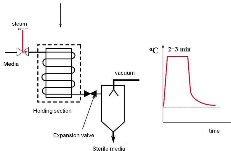
Fig. 4.148: Steam injecting continuous culture media sterilizer
