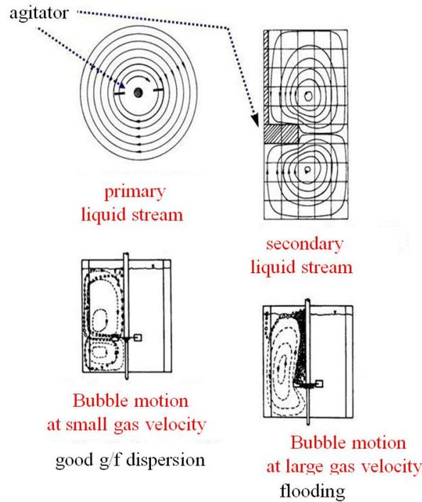
Fig 4.86.: Primary and secondary fluid streams and bubble movement in agitated reactors
