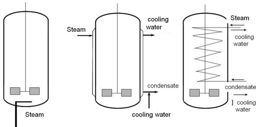
Fig. 4.147: Heating, cooling solutions
