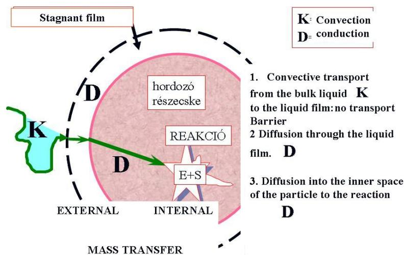
Fig 2.65.: Mass transfer resistances on and in a particle
