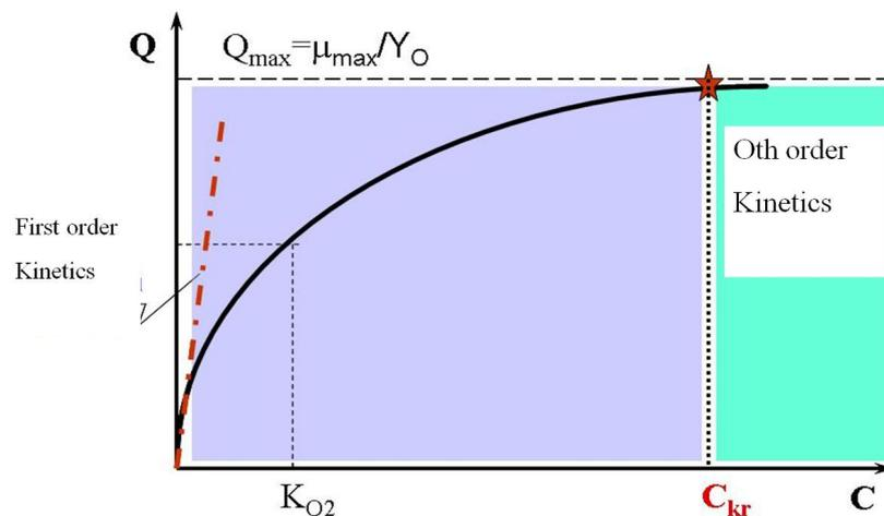
Fig 4.72.: Specific respiration rate as a function of dissolved oxygen concentration.
