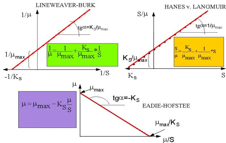
Fig 4.7.: Monod-model, graphical methods to evaluate  $K_S$  and  $\mu_{\max}$ .
