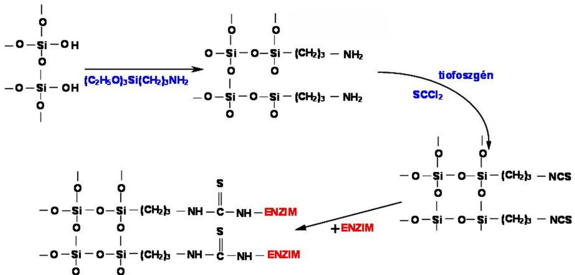
Fig 2.58.: Immobilization onto glass surface
