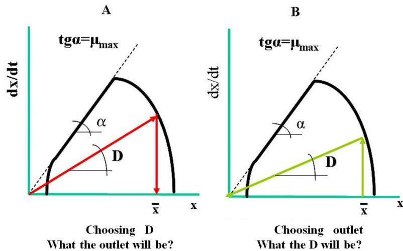
Fig 4.52.: Designing a chemostat with a graphical method
