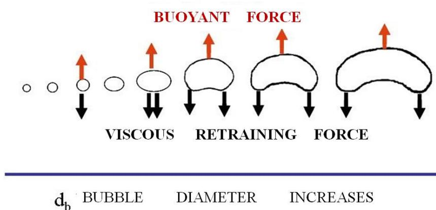
Fig 4.81.: Deformation of the bubble shape with the increasing diameter
