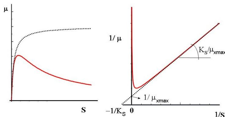
Fig.4.27.: Substrate inhibition
