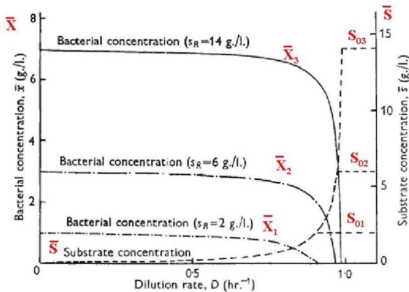
Fig 4.44.: Dependence of steady states on inlet substrate concentration.
