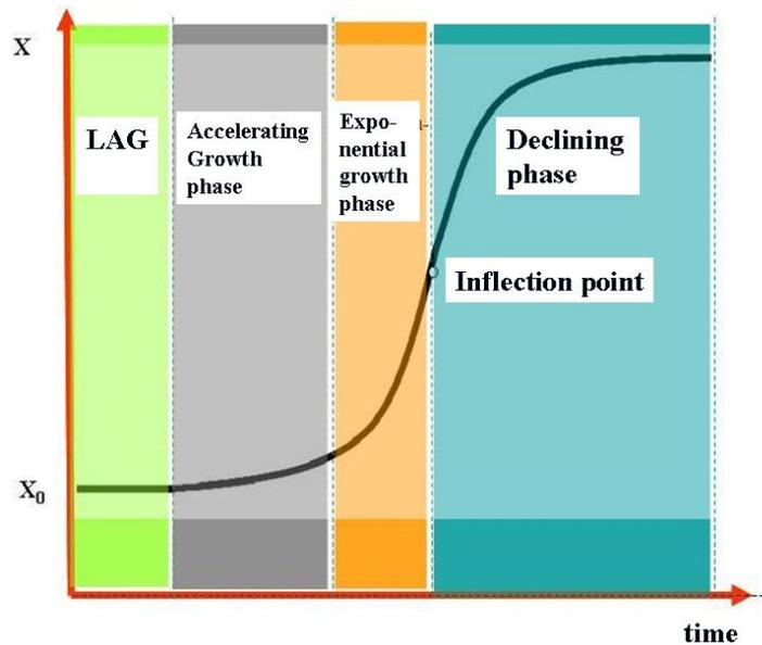
Fig 4.2.: Batch fermentation's real growth curve
