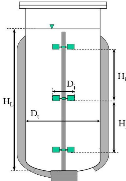
Fig 4.85.: Bioreactor with more mixing devices
