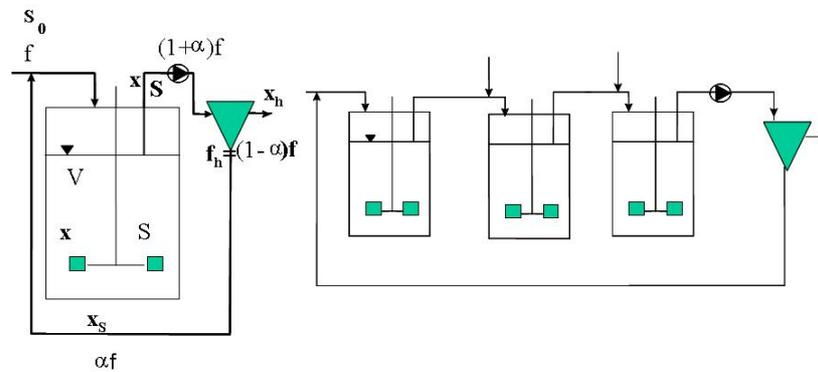
Fig 4.56: Cell retention and recycle
