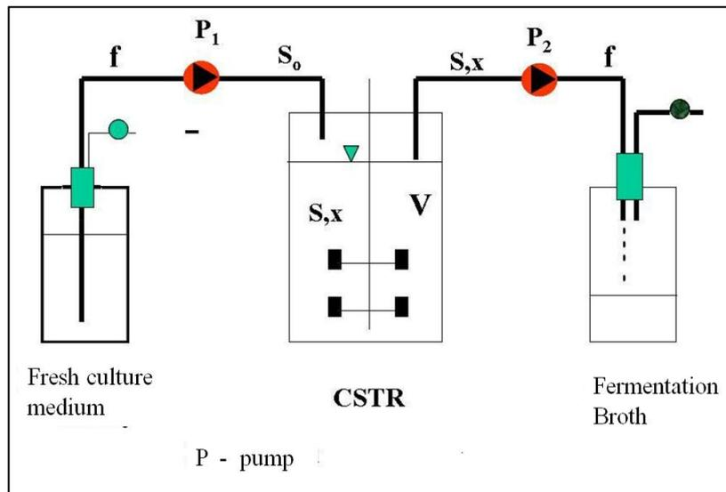
Fig 4.42.: Chemostat continuous fermentation setup
