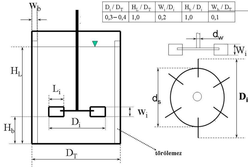
Fig 4.84.: Main geometrical ratios of the standard fermentor
