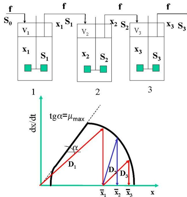
Fig.4.54.: Single stream multiple stage continuous system
