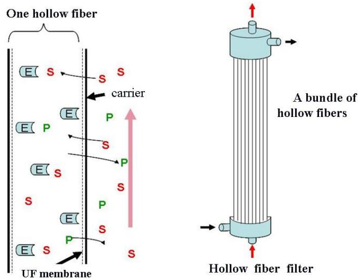
Fig 2.64.: Hollow fiber, UF membrane
