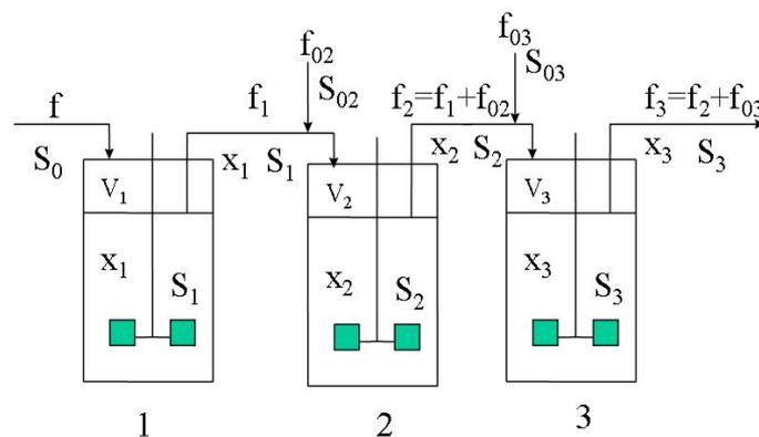
Fig 4.55.: Multistream multistage chemostat
