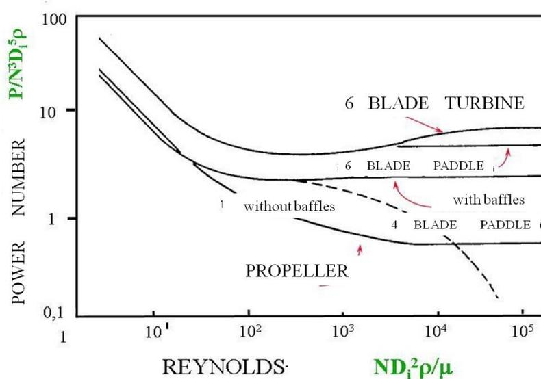
Fig 4.87.:  $N_p$ - $Re$  plot for different impellers (Newtonian fluids)
